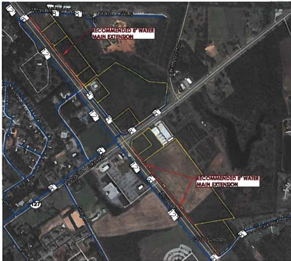
Figure 5 – Recommended Water Improvements
