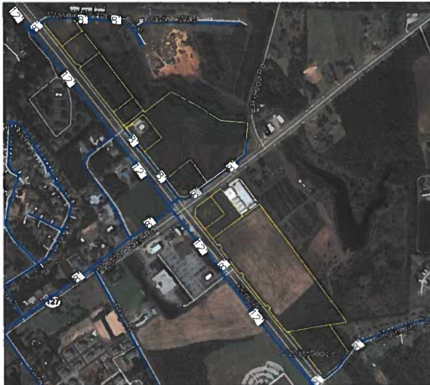
Figure 3 – Existing Water System in Study Area
