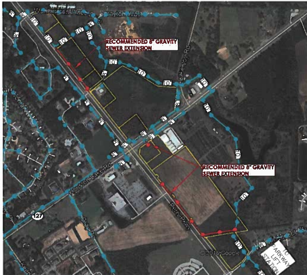
Figure 4 – Recommended Sewer Improvements
