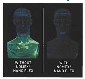
FAST UV-light photographs without Nomex® Nano Flex (left) and with Nomex® Nano Flex (right) illustrating after particle exposure for the test subject's head and neck; bright yellow areas show where particles penetrated the ensemble.
