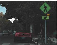
**Flashing Sign Beacon** – A flashing beacon assembly used to highlight a regulatory sign or warning sign. Red flashing beacons can be used to enhance the visibility or conspicuousness of a stop sign in order to achieve better motorist compliance of the stop condition. Yellow flashing beacons can be used to emphasize potentially unexpected or hazardous conditions conveyed by various types of warning signs.
